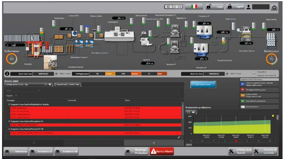
1. Movicon.NEXT screen representing the Container Filling Line graphically
